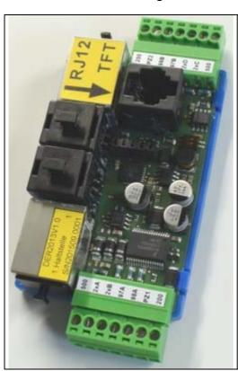
The remote station ER-2013 provides 8 inputs and outputs, including 6 free inputs and outputs. There are 2 piezo-buzzer-outputs for the call messaging of bus-matrix-indicator.
