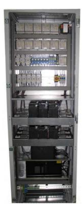
Coloured control cabinet KW07: 1800 x 600 x 400mm (H x W x D) at IP54. Control cabinet mounting plate and the contactor plate are mounted for protection against oscillation. Control cabinet with integrated air filter box with thermostatically controlled fan. Optionally there is a air codition system available.
