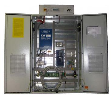
Coloured control cabinet KW06: 1200 x 1000 x 350mm (H x W x D) at IP54. Control cabinet mounting plate and the contactor plate are mounted for protection against oscillation. Control cabinet with integrated air filter box with thermostatically controlled fan. Optionally there is a air codition system available.
