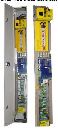
MRL Roomless Controler Frequency Inverter Rope / Hydraulics Casing KW 240 Coloured control cabinet KW240: 2000 x 240 x 220mm (H x W x D) for roomless elevators (MRL) for mounting in / or beside the shaftdoor.
